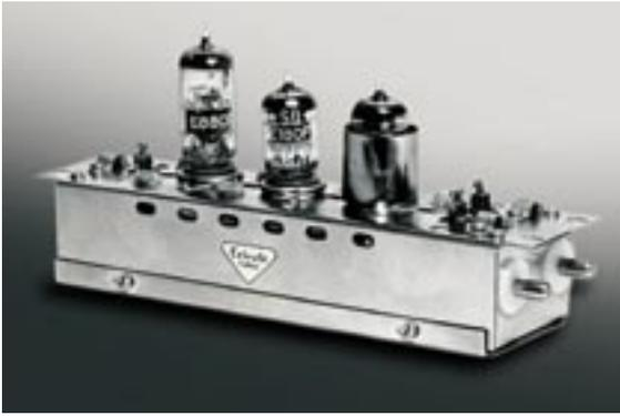
**Naturally, the first antenna amplifiers** used electron tubes. Teleste was also among the first to apply the new transistor technology when it became available.
