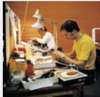
**Teleste's master aerial devices** were modular from the very beginning. In the early 70's, sound devices started to be built using a similar structure – the D series (Domino) included a large amount of various types of plug-in units. The modular structure of products made Teleste a flexible supplier. Manufacturing was done mainly by hand and there was little subcontracting.
