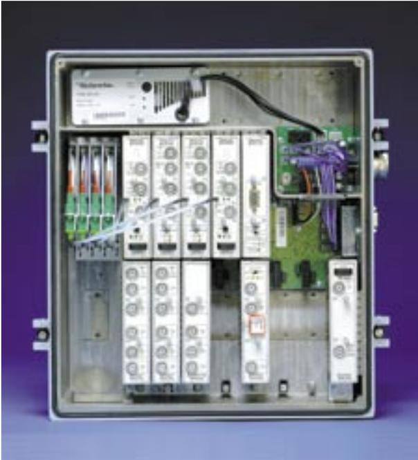
**BXX, the modular intelligent optical node**, was developed in the mid-'90s for the new generation cable television networks to support two-way pay-TV and cable modem services. The first significant client was Telenet and Interelectra in particular.
