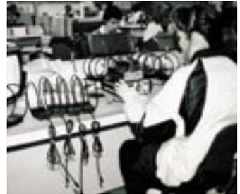
**Assembling a Super Loop aerial at the Ealy plant.** The aerial included Teleste's first application-specific integrated circuit (ASIC), which detected whether the TV set was turned on and activated the aerial amplifier accordingly.
