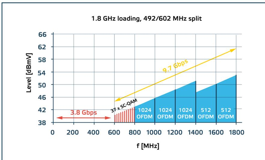
**Figure 7:** Throughput, RPD Node and three cascaded amplifiers
