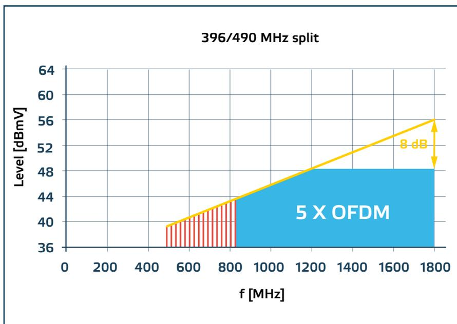
Figure 3: An example load leading to 70 dBmV TCP
