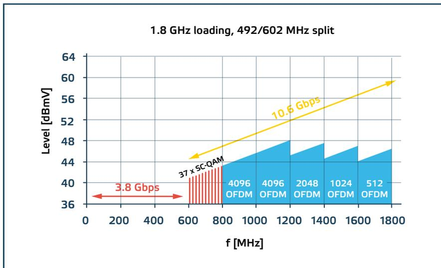
Figure 8: Throughput, RPD Node and four cascaded amplifiers
