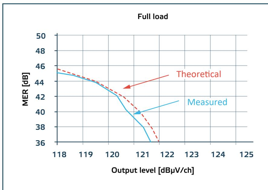
Figure 4: Three cascaded amplifiers, theoretical MER versus measured MER
