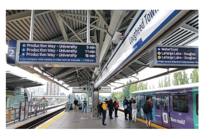
conditions is guaranteed by the internal thermal management system, which ensures that the operating temperature stays between the temperature range from -35  $^{\circ}$ C to +55  $^{\circ}$ C. The intelligent diagnostic unit with versatile features monitors display performance and operations in real time.
